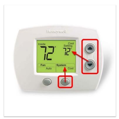
The Fan is usually on Auto, but you can change the System from Cool to Heat using the button underneath it. Use the Arrows to choose the desired temperature.
